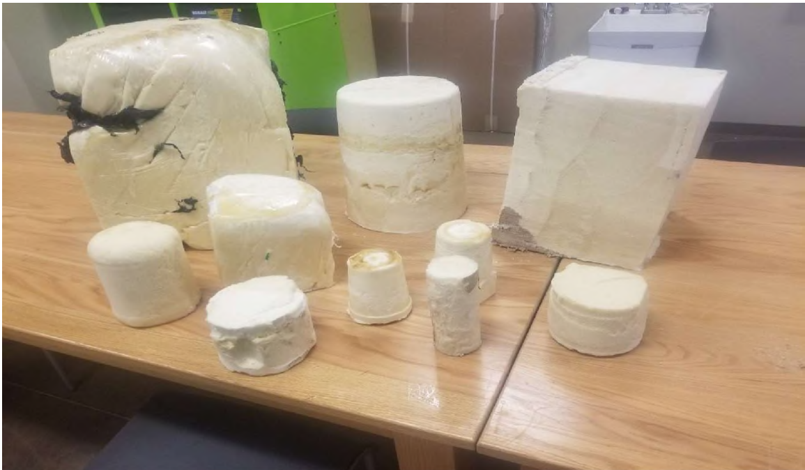
Figure 2.5. Ten rigid polyurethane foam blocks cast with variable dimensions used for volumetric confinement analysis.
