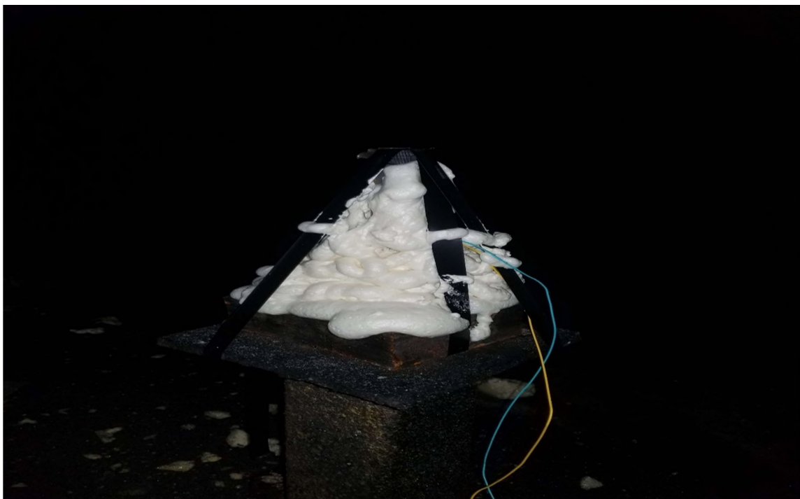
Figure 2.4. Confinement test of TexPak 10-minute foam cure time.
